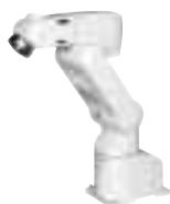
Vertical articulated robot RV Series
